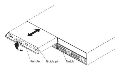
Figure 42. Removing and replacing controller A
